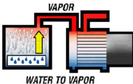
A high vacuum pump is capable of removing all moisture from a hermetic system by reducing internal system pressures to the boiling point of water at normal temperatures. For those being introduced here to high vacuum work, it should be stated that a vacuum pump does not “suck out” the liquid moisture, but rather causes it to boil in to a vapor state which can be harmlessly removed from the system and exhausted through the vacuum pump.
